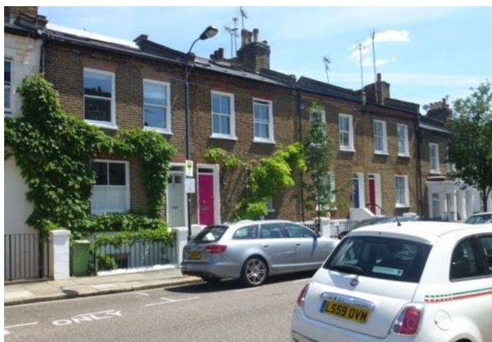
Nasmyth Street – flat fronted cottages in the foreground, canted ground floor bay windows in the group beyond.
